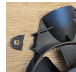
Cooling fan mounting – before repair
