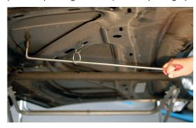
It is not always possible to locate a suitable place from which to hang the S-hook; in this case choose a suitable (strong) part of the surrounding bodywork and protect with suitable padding.
